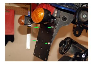
Install the turn signal/taillight plate. Leave the wires hanging; do not install the reflector as shown in the following photo. Install it as shown using the 4mm Allen and 10mm lock nuts.
