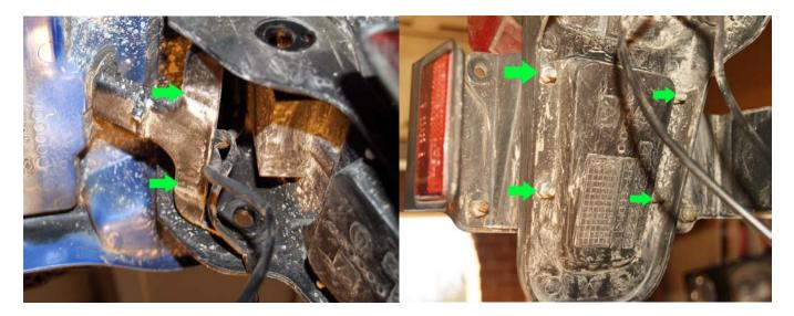
Once both signals are disassembled, fish the wires through the original mounting holes and clip the two zip-ties holding the wires for the turn signals in place.
