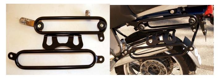
Install the left main mounting bracket as shown. It bolts up identically to the right side.
