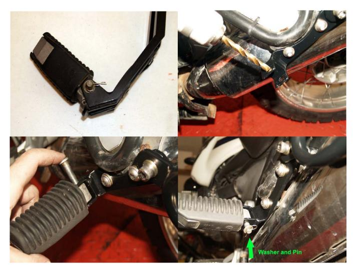
On the foot pegs, you should need no tools, unless the pins won't fit in the holes for the pegs, in which case you would use a drill, or round file, to clean some of the powder coat out to fit the pins.
