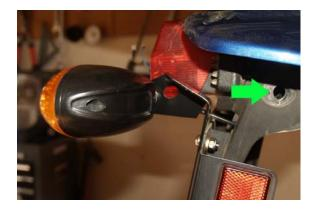
To stiffen the original mount you can reinstall the signal stalks in the original holes, or use similar sized bolts and nuts with washers to connect the two parts.
