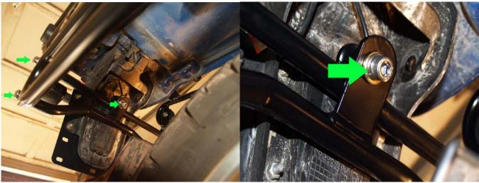
Install the two rear support brackets to the left and right main mounts as shown. Bolt the upper and lower support brackets to each other. Snug down all five bolts (three showing, the other two on the left main bracket), ensuring they all contain the washers that came with them.
