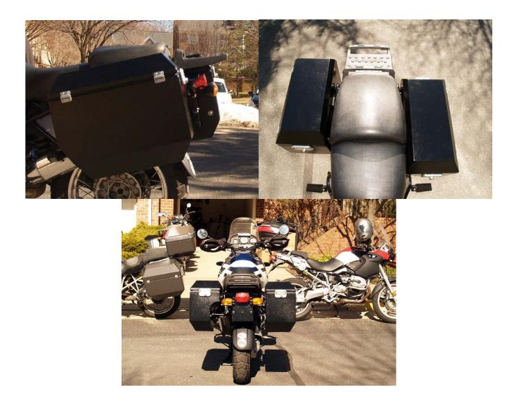
Remember, these bags are designed to be moved on the mounts. They will move as much as 3 inches for and aft. Depending on your needs, you can adjust them to suit. They will need to be completely removed and repositioned for this adjustment.
