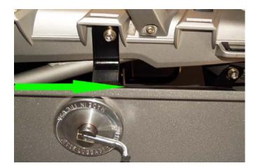
Angle the bag by grasping it end to end and make sure it is level with the mounting bars on top. See arrow on this and previous page.
