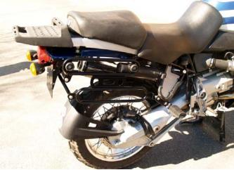
Install the bracket loosely as shown in the above photos with a 5mm Allen.
