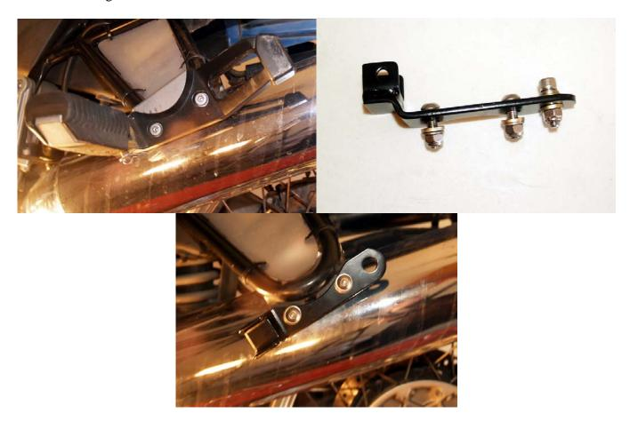
Remove the left side foot peg bracket with a 5mm Allen. Prepare the replacement foot peg bracket by removing the bolts and nuts in the photo above. Install and add locking nuts as shown.
