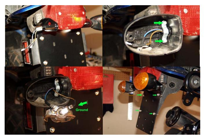
Installing the lights is the reverse of removal, except leave out the signal stalks. Attach the signals to the license plate bracket.
