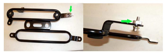
Left is the right side main bracket with the attached hardware. Right, note the hardware and spacers, they are in the correct positions.
