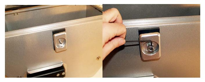
Peal off the protective covers on the composite block tape strips, place over the hole in the bag as shown. Push the crank handle shaft through the hole and thread on the cam. Add the supplied washer next. Use the supplied Allen to tighten the setscrew. Repeat on the other side bag. Keep the lower mounting plates loose for now.
