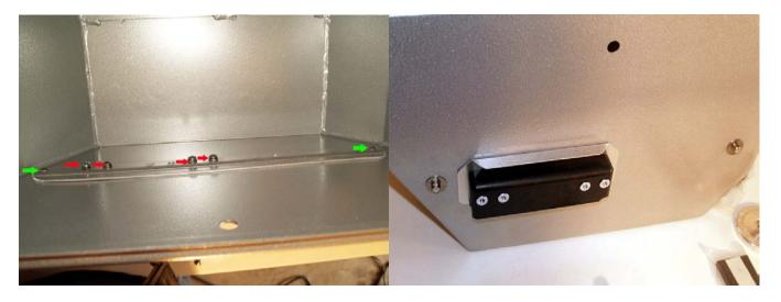
Install the long bolts (4) (left) with a lock washer (split washer) then a flat washer and through the bag into the metal plate and threaded composite block (right). Keep these loose for now.
