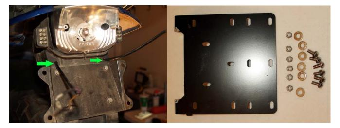
Allow the wires to hang down beside the taillight. They will be fed through the mounting bracket later.
