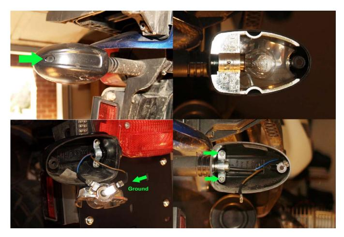
Pull the turn signals apart: Remove the Phillips screw, and then gently pull the lens off. Inside you pull the chrome reflector out straight; you may need to gently pry it. Once out, disconnect the wires, and remove the reflector.
