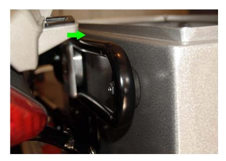
Use the crank handle to rotate the mount cam until it covers the upper mounting bracket on the bike. Until you have it properly adjusted, it may need to be turned by hand on the mounting cam. Do not tighten it yet.
