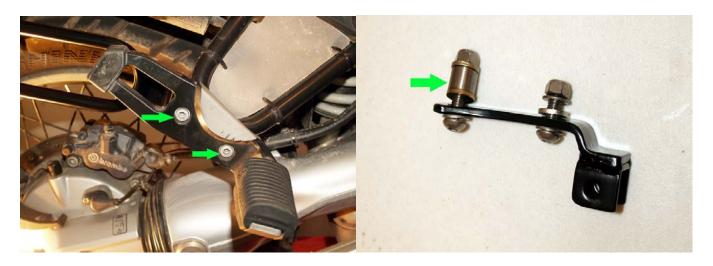
Remove the right foot peg bracket with a 5mm Allen (left). Install the replacement bracket (right) with the washers and spacers as shown. First use the bolts to thread the bracket in place and firmly snug them down with a 5mm Allen. Then add the spacers and connect the rear bolt to the main mounting bracket with the large spacer, see photo (bottom right) on the previous page. Add the 13mm nuts and washers to both bolts and tighten them.
