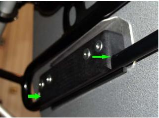
Make sure the lower composite block is fully seated on the lower mounting bracket. See arrows.
